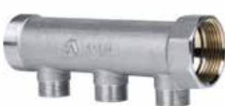
Collettore 3 vie M/F cromato derivazioni interasse 50 mm. Attacco 24x19 sistema intercambiabile per tubo rame, plastica e multistrato fino Ø20. 3 ways chromium-plated manifold M/F center distance connections 50 mm. Connection 24x19 interchangeable system for copper, plastic and multilayer pipe up to Ø20.
