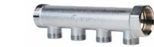
Collettore 4 vie M/F cromato derivazioni interasse 50 mm. Attacco 3/4 maschio eurocono. 4 ways chromium-plated manifold M/F center distance connections 50 mm. Connection 3/4" male eurocone.
