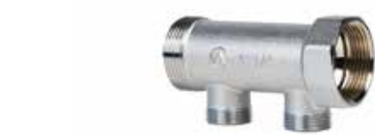
Collettore 2 vie M/F cromato derivazioni interasse 50 mm. Attacco 3/4 maschio eurocono. 2 ways chromium-plated manifold M/F center distance connections 50 mm. Connection 3/4" male eurocone.
