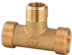
Raccordo a “T” maschio in ottone giallo con due attacchi tubo rame, plastica e multistrato. Yellow brass male tee fitting with two connections for copper, plastic and multilayer pipe.
