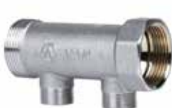
Collettore 2 vie M/F cromato derivazioni interasse 50 mm. Attacco 24x19 sistema intercambiabile per tubo rame, plastica e multistrato fino Ø20. 2 ways chromium-plated manifold M/F center distance connections 50 mm. Connection 24x19 interchangeable system for copper, plastic and multilayer pipe up to Ø20.
