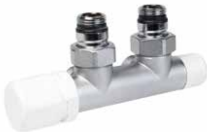
Valvola BITUBO termostattizzabile, interasse 50 mm, senza by-pass versione sinistra. Left double pipe radiator valve, centre distance 50 mm, with thermostaic option without by-pass.
