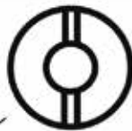
By-pass chiuso Closed bypass
