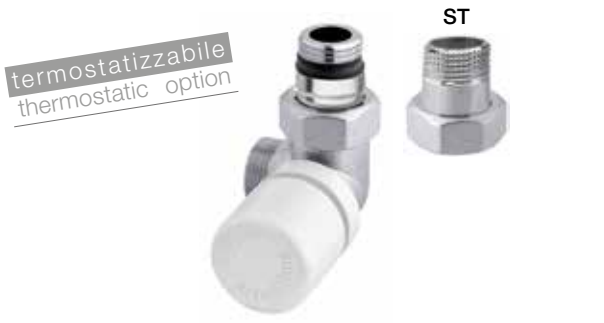
Valvola termostattizzabile cromata ad angolo, versione destra. Attacco tubo rame, plastica e multistrato. Chromium-plated right angle radiator valve with thermostatic option. Connection for copper, plastic and multilayer pipe.
