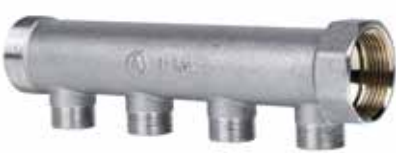
Collettore 4 vie M/F cromato derivazioni interasse 50 mm. Attacco 24x19 sistema intercambiabile per tubo rame, plastica e multistrato fino Ø20. 4 ways chromium-plated manifold M/F center distance connections 50 mm. Connection 24x19 interchangeable system for copper, plastic and multilayer pipe up to Ø20.
