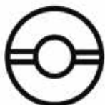
By-pass aperto Opened bypass
