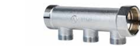
Collettore 3 vie M/F cromato derivazioni interasse 50 mm. Attacco 3/4 maschio eurocono. 3 ways chromium-plated manifold M/F center distance connections 50 mm. Connection 3/4" male eurocone.
