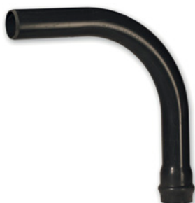
3003 CURVA LARGO RAGGIO A 90° CON O-RING PN 10 / 90° WIDE RADIUS BEND WITH O-RING PN 10 / COURBE MF GRAND RAYON 90° PN10
